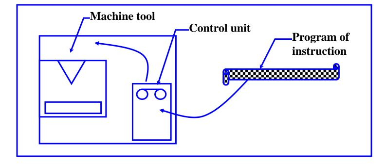
**The program of instruction** is a numerical or symbolic code that is detailed step-by-step to tell the machine tool what to do.
